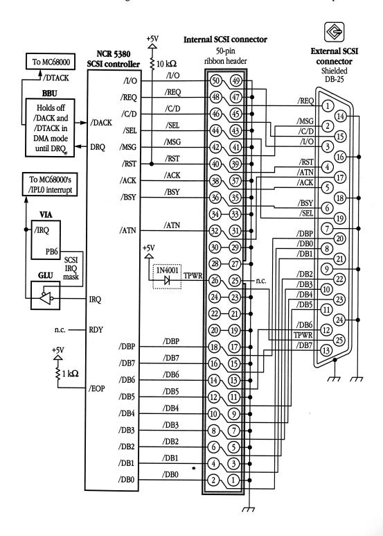
■ **Figure 11-6** Circuit diagram of the SCSI interface on the Macintosh Portable computer
