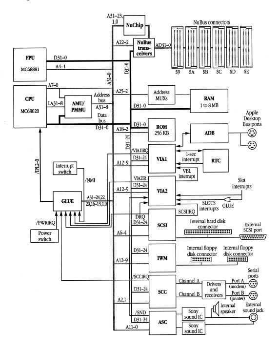
■ Figure 2-7 Block diagram of the Macintosh IIx and Macintosh IIcx computers
