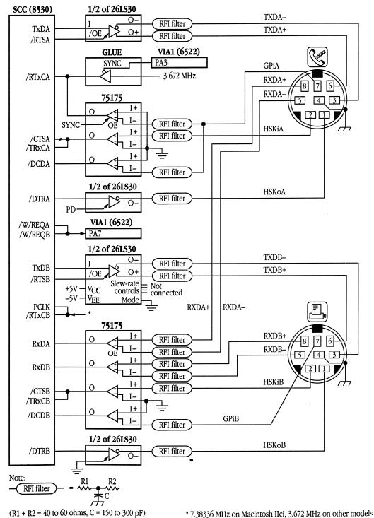
grown Vilon orange Green ■ Figure 10-6 Circuit diagram of the serial I/O interface in the Macintosh IIfx computer
