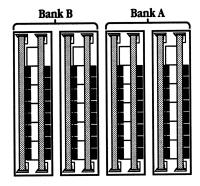
System memory size: 8 MB Bank A: four 1 MB SIMMs Bank B: four 1 MB SIMMs
