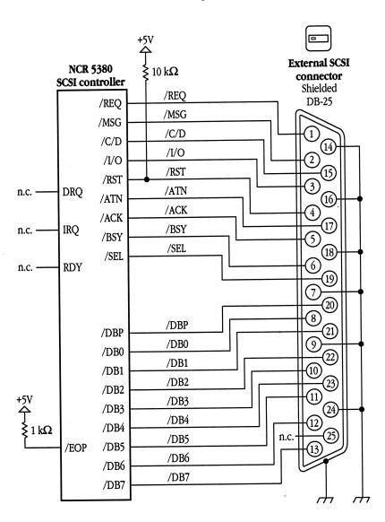
■ **Figure 11-5** Circuit diagram of the SCSI interface on the Macintosh SE computer
