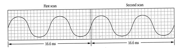
You can perform your own updates of the sound buffer using the vertical blanking interrupt from the VIA to synchronize your updates to the buffer scan. For the sake of compatibility with different models, Apple recommends that you use the routines in the Sound Driver and the Sound Manager to generate complex sounds.
