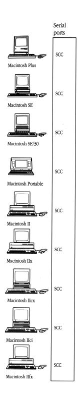
The Macintosh serial interface is controlled by a Zilog Z8530 Serial Communications Controller (SCC) integrated circuit. The SCC provides two serial ports: SCC port A—the modem port—and SCC port B—the printer port. Each SCC port has a connector, located on the back panel, for connecting serial peripheral devices and for connecting the computer to the AppleTalk network.
