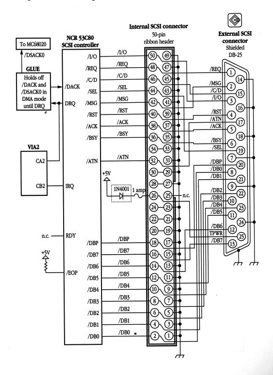
■ Figure 11-8 Circuit diagram of the SCSI interface on the Macintosh SE/30, Macintosh IIx, Macintosh IIcx, and Macintosh IIci computers
