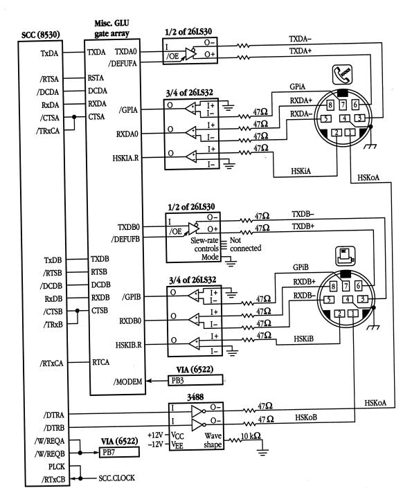
■ **Figure 10-5** Circuit diagram of the serial I/O interface in the Macintosh SE/30, Macintosh II, Macintosh IIx, Macintosh IIcx, and Macintosh IIci computers
