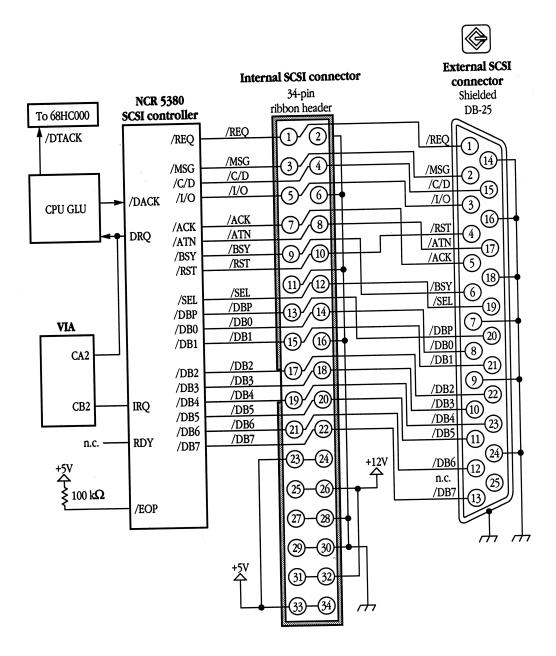
■ Figure 11-7 Circuit diagram of the SCSI interface on the Macintosh II computer
