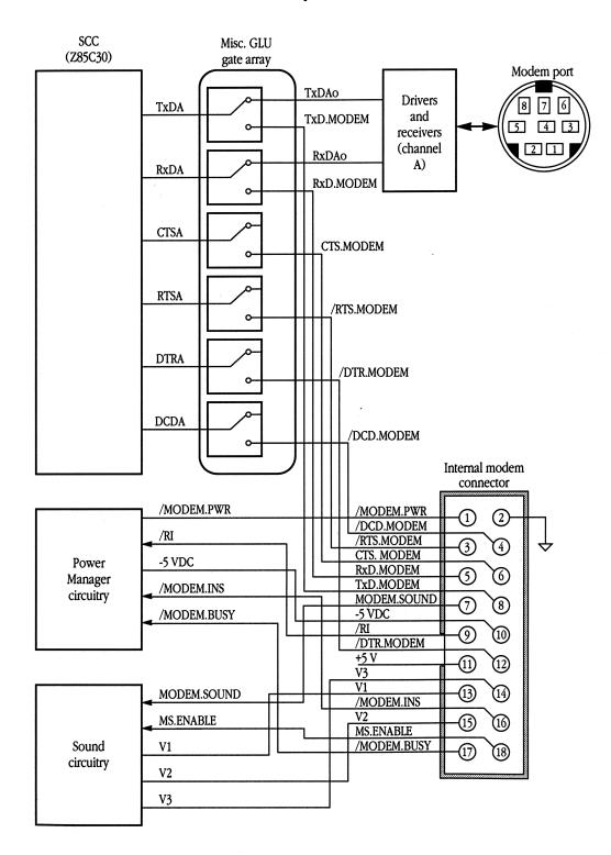
■ **Table 10-3** Signal assignments for the modem connector in the Macintosh Portable computer
