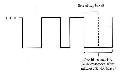
A device sends a Service Request signal repeatedly until it receives a command from the computer. When a device requests service, the computer does not know which device sent the request. Therefore, the computer polls each of the devices by sending a Talk Register 0 command, beginning with the last active device. Only a device that has data to send responds to the Talk command.
