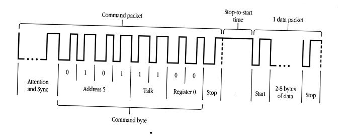
Two signal lines from the VIA to the transceiver—ST0 and ST1—define the ADB transaction state, which controls the sequence of operations performed by the ADB transceiver chip. After each part of an ADB command transaction is complete, the computer uses lines ST0 and ST1 to advance the ADB transceiver to the next transaction state, ready for the next part of the communication. There are four possible ADB transaction states, as shown in Table 8-12.
