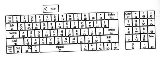
Notice that these response codes are not all the same as the key codes returned by the Keyboard Driver software. The standard 'KMAP' resource supplied in the System Folder reassigns several key codes, as shown in Table 8-6.
