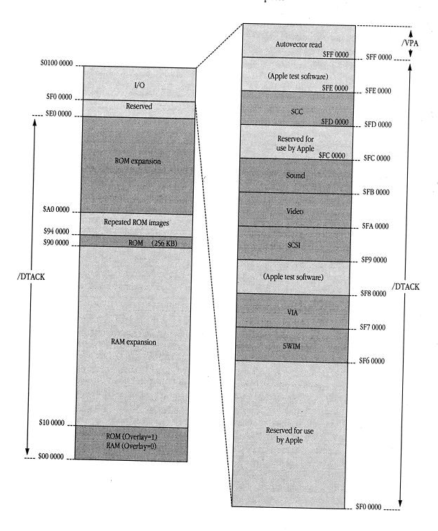
When the main processor receives an interrupt, it performs a read operation with all address lines set to 1 except A3 through A1; lines A3 through A1 reflect the level of the interrupt. When the CPU GLU receives an address in the range \$FF 0000 to \$FF FFFF, it asserts /VPA, which causes the main processor to jump to the location in memory containing the appropriate interrupt handler. Interrupts are discussed in the section "MC68000 Interrupts," earlier in this chapter.
