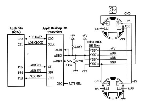
■ Figure 8-3 Circuit diagram for the ADB interface on Macintosh II, Macintosh IIx, Macintosh IIcx, and Macintosh IIci computers
