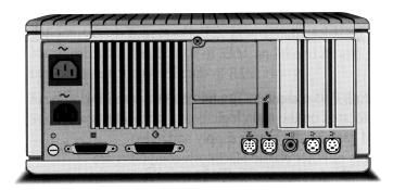
Figure 1-13 shows a back view of the Macintosh IIci computer. Notice the addition of a connector for a video monitor.
