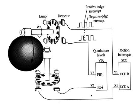
A rubber-coated steel ball in the mouse turns as the mouse is moved and contacts two capstans, each connected to a slotted wheel called an *interrupter wheel*. Motion in the mouse's X-axis direction (left and right) rotates one of the wheels and motion in the Y-axis direction (up and down) rotates the other wheel.
