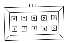
Table 6-5 shows the signal assignments for the connector from the power supply to the logic board in the Macintosh IIcx and Macintosh IIci computers.
