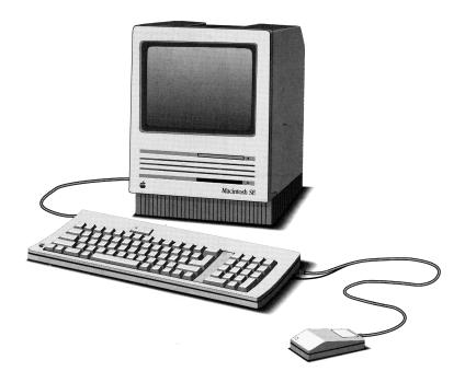
Figure 1-5 shows a front view of the Macintosh SE/30 computer. Notice the video screen, disk drive access opening, keyboard, and mouse.
